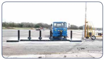
and two fixed bollards to accommodate access for large vehicles or tight turning circles has also succeeded in its PAS68 crash test, halting a 7.5 tonne truck travelling at 64 kph (40 mph).
